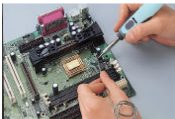
Function as soldering iron ~ 500°C (20 – 60 Watts)
